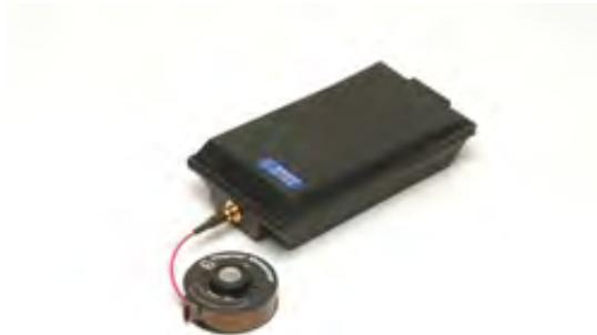
The Hagner EC1-X UV-C Digital Radiometer is of the same type as EC1-X UV-A above but measures UV-C radiation at 253.7 nm over a range of 0.001 - 2,000 W/m<sup>2</sup>.
