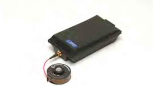
The Hagner EC1-X UV-B Digital Radiometer is of the same type as EC1-X UV-A but measures UV-B radiation (265 - 370 nm) over a range of 0.001 - 2,000 W/m<sup>2</sup>. NB: In order to cover the important wave length 310 nm, the detector also has a sensitivity in the UV-A range .
