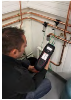
DHW network temperature
